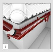
Internal/external corners (KIB/ KEB) are fixed through bonding with the help of the gutter joint (BJ) and the gutter joint element (EJ).
