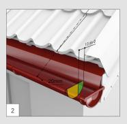
It is recommended to mount the gutter so that its outer side is 20-30 mm lower than the imaginary extension of the roof structure. Thus, the flow of water from the roof will not go over the gutter.
