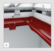
Two gutters that are to be joined should be placed on the hooks without being fixed. The distance between the edges of the gutters should be approximately 2-3 mm.
