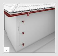
Pipe holders (BB) are fixed on the wall one under the other with dowels before the pipes (BU) are installed. The maximum distance between two BB should not exceed 2 meters \*\*\* (the BB calculation can sometimes not meet your requirements. Calculate the amount of BB for each drainage).
