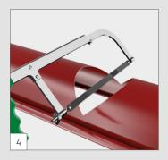
Mark a spot and use a saw and tinsnips to cut a drainage slot in the gutter, which should not be larger than the diameter of the pipe.
