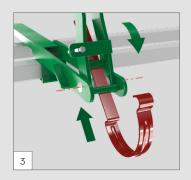
Before you mount the hooks (CJ), you should bend them so they match the angle of the roof inclination with a special device, according to the drainage slope
