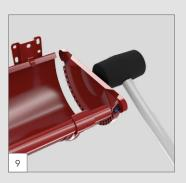
The universal stop (CU) end is fixed manually or using an elastic hammer at the end of the gutter, without using silicon because it destroys the gasket through time.
