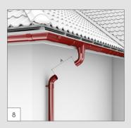
Pipe bends 60° (CB) are mounted on the gutter outlet (RA) and down onto the pipe (BU). They can be joined through the intermediate pipe (PB). Measure the distance between the bends "a", add 100 mm to it, for both ends of the intermediate pipe, each of which enter the bends by 50 mm.
